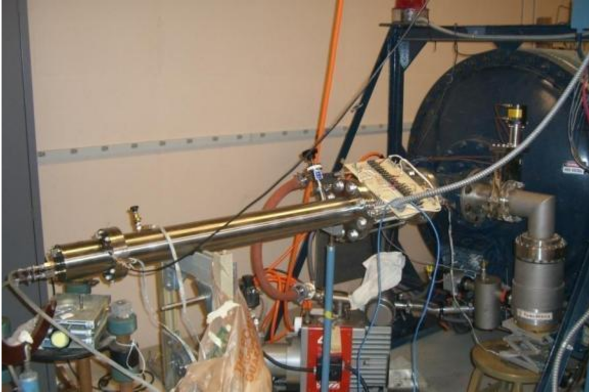
Figure 19. Picture of the Dynamitron with the cold head attached to the end of the beam line. The cold head is electrically isolated and pumped to a vacuum level of 10^{-7} torr. Water flows through the cold head to maintain the samples at a constant room temperature.
