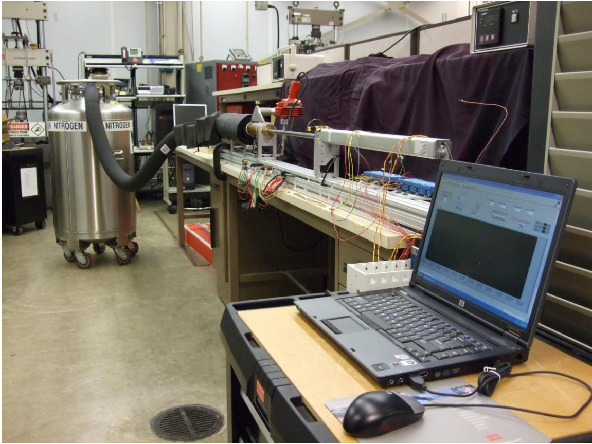
Figure 22. Picture of the thermal cycle apparatus used to simulate the space thermal environment.
