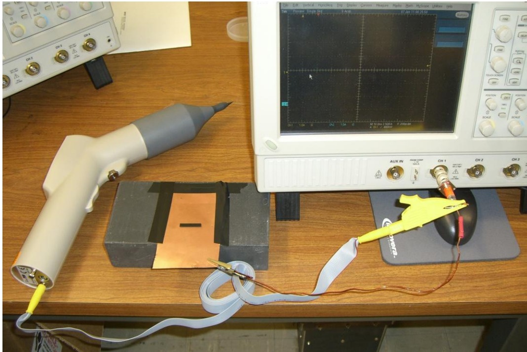
Figure 13. ESD test setup showing the ESD3000 discharge source, sample under test, SDN-414-025 current viewing resistor, tektronix Oscilloscope, cooper wire, copper plate and rubber brick.
